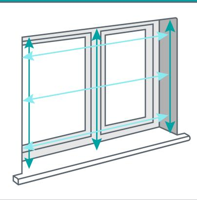
First, measure across the top, middle and bottom of the recess (the horizontal arrows shown). Ensure you measure from edge to edge of the whole window recess. When ordering your blind, please provide us with the smallest of these 3 measurements.
