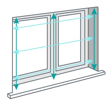
First, measure across the top, middle and bottom of the recess (the horizontal arrows shown). Ensure you measure from edge to edge of the whole window recess. If you plan to fit your blind towards the back of the recess (nearest the window), make sure you take your measurements from here. When ordering your blind, please provide us with the smallest of these 3 measurements.
