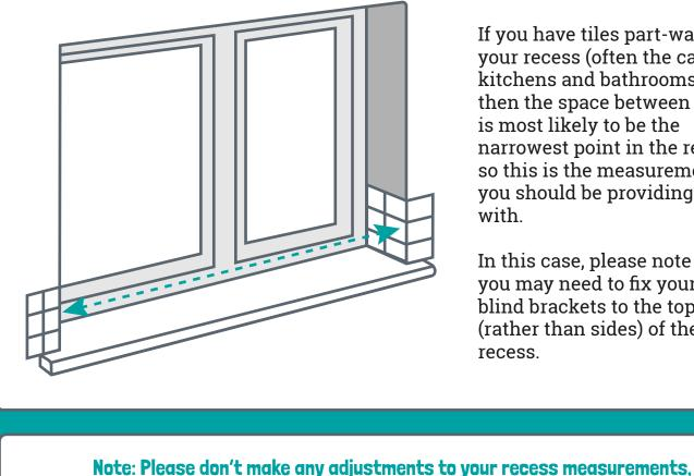
your recess (often the case in kitchens and bathrooms) then the space between them is most likely to be the narrowest point in the recess, so this is the measurement you should be providing us with. In this case, please note that
